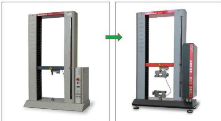
Picture 6: ProLine 2010 with MOPS electronics before modernization
